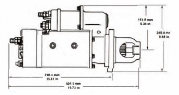
The 42MT is a straight drive starter for heavy duty applications available in 12 Volt and 24 Volt configurations. The 42MT features a Semi Solid Link solenoid and optional Over-Crank Protection.
