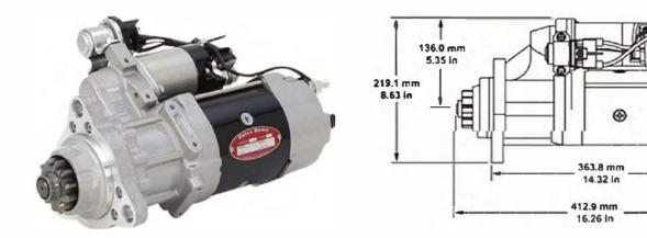
The 39MT is a gear reduction starter ideal for heavy duty truck and off highway applications. The drive has an electrical soft start that rotates the pinion for proper ring gear engagement before cranking, minimizing tooth abutment related damage. The sealed solid link solenoid eliminates contact welding in low system voltage situations, providing enhanced reliability. Sealed noseless configuration minimizes debris accumulation and contamination reducing maintenance expense.
