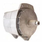
System voltage: 24 Volt Output: 150 A Mounting style: J180 Rotation: clockwise Housing coating: RAW Mounting bolt size: .505-.520 Mounting ear size: 1/2-13 Mounting holes: 3 Positive stud size: 5/16-24 Negative stud size: 1/4-28 Rectifier location: internal Shaft diameter: 7/8 inch Regulator locationIntegral Regulator number: 8RL3136 Weight: 14 kg
