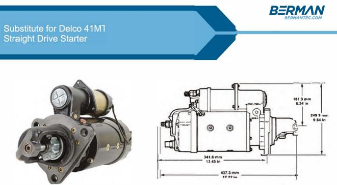
The 41MT is a straight drive starter for heavy duty applications rated at 5.0 kW for 12 Volt applications and 7.0 kW for 24 Volt applications.
