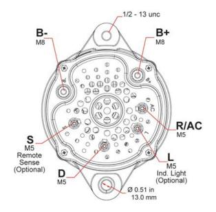
If the vehicle has an ignition (excite) circuit, connect wire to "D" (dummy) terminal.
